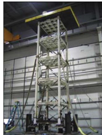
Figure 2. Rocking truss pier specimen on 6DOF shake table.
